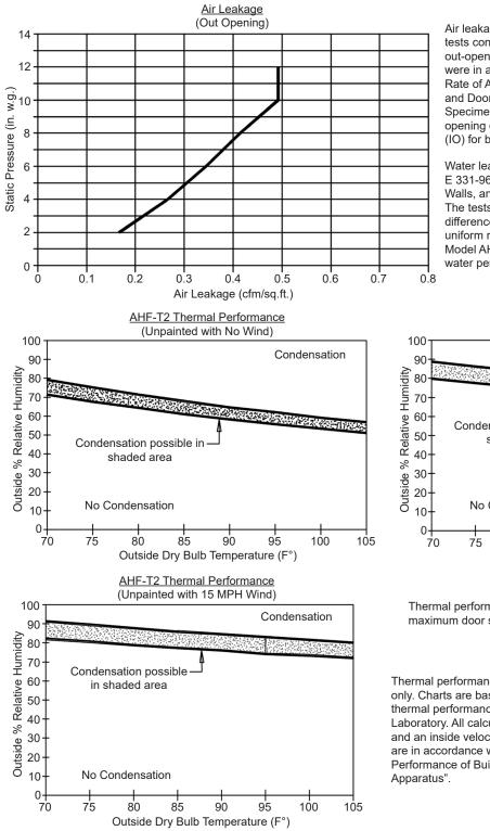
Air leakage chart is based upon independent air leakage tests conducted by Architectural Testing Laboratory. The out-opening model of a 26" x 60" AHF-T2 was tested. Tests were in accordance with ASTM E 283-91 "Determining the Rate of Air Leakage through Exterior Windows, Curtain Walls, and Door under Specified Pressure Differences Across the Specimen". Louvers & Dampers recommends using out of opening doors for draw through applications and in opening (IO) for blow through applications.
