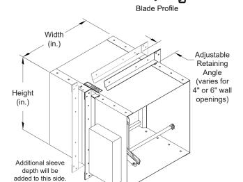
\*Dampers smaller than minimum frame size require a transition. Reference SD-TRFS. Dampers less than 6"H will have a 20" sleeve with the additional sleeve length on the jackshaft side when a B-Pan type transition is ordered.
